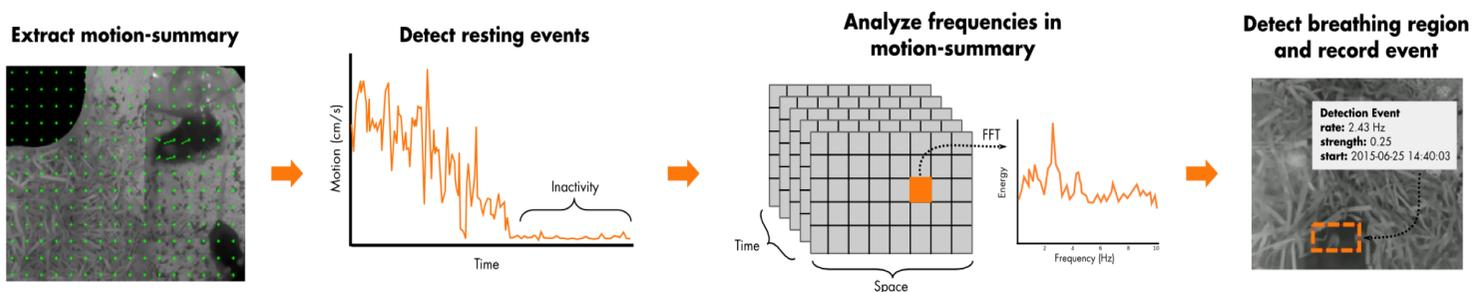
Figure 1: Breathing rate is generated from HD video using computer vision algorithms.
