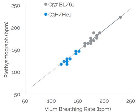
Figure 2: Breathing rate generated from the algorithm is highly correlated to breathing rate measured using the conventional plethysmograph.
